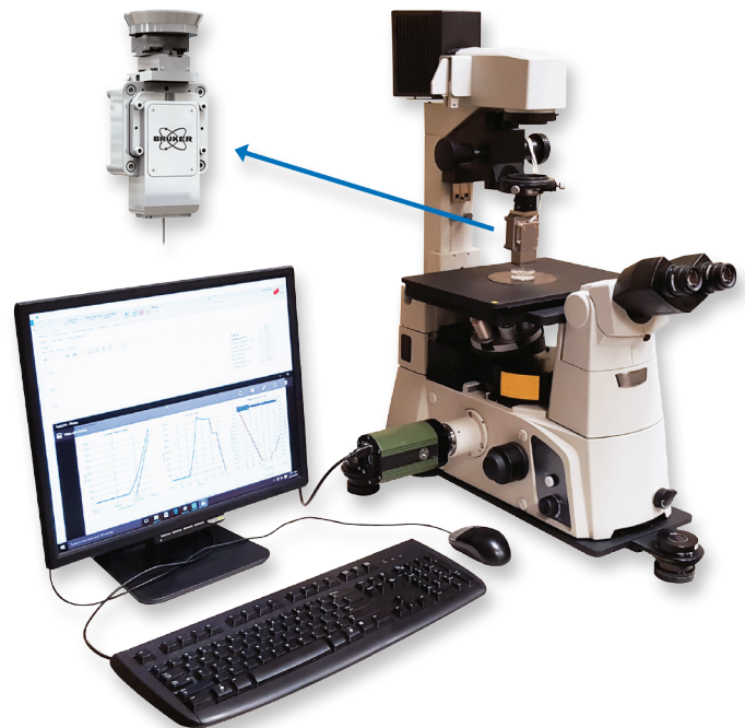
Figure 1. Hysitron BioSoft In-Situ Indenter performing testing while attached to an inverted microscope.
